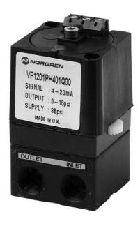
Electrical connection: Screw terminal Port sizes: 1/8" BSP/NPT Command signal: 4 to 20mA or 0 to 10V Electrical supply: 24V d.c.  $\pm 10\%$  (on 3 wire options) Loop resistance: mA = 220  $\Omega$  maximum, V = 16 k $\Omega$  minimum Failure mode: Fails safe upon loss of signal or power
